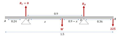
Equations with unknown distance, x, measured from C
